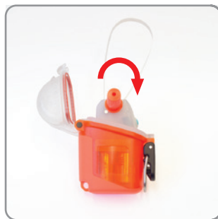
Insert the tool and antenna into the round open space in the back of the top cap.
