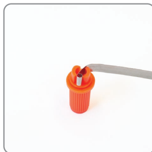
To rewind the antenna, use the tool provided in the box.
